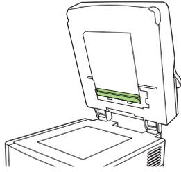
4. Clean the ADF backing and the calibration strips by wiping them with a clean, damp, lint-free cloth. Use an ammonia-based surface cleaner to dampen the cloth.
