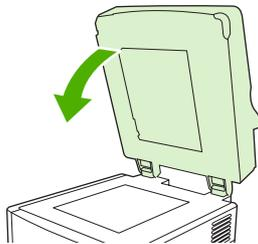
5. Push the release button to open the ADF cover.
