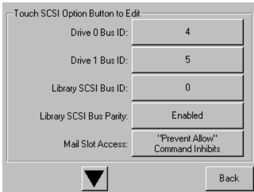
Figure 20 SCSI option selection screen (two-drive model shown)
