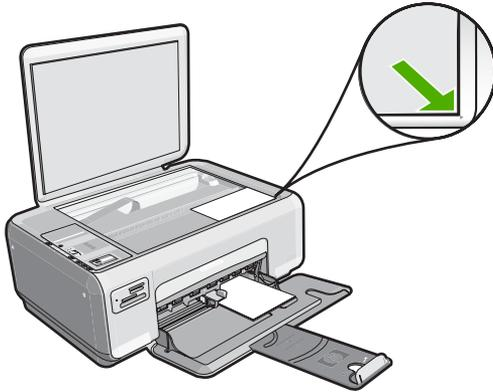
**Cause:** Debris might be stuck on the glass or on the back of the document lid. The HP All-in-One interprets anything it detects on the glass as part of the image.
