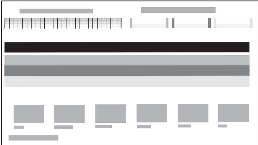
3. Make sure the test patterns show a complete grid and the thick color lines are complete.
