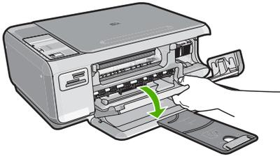
4. Wait until the print carriage is idle and silent, and then lightly press down on a print cartridge to release it.
