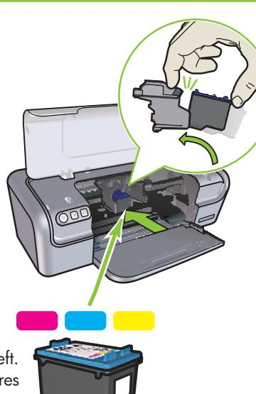
A black print cartridge is not included with your printer. It is not required to operate the printer.
