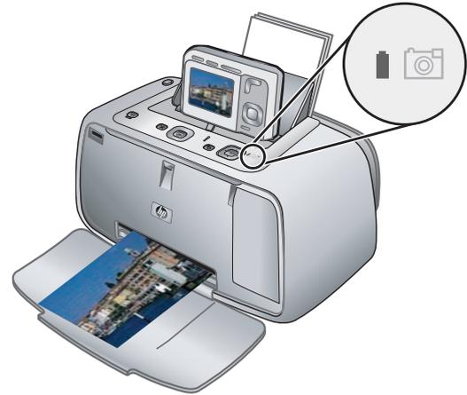
1. Place a few sheets of HP Advanced Photo Paper in the input tray with the glossy side facing the front of the printer and adjust the paper-width guide.
