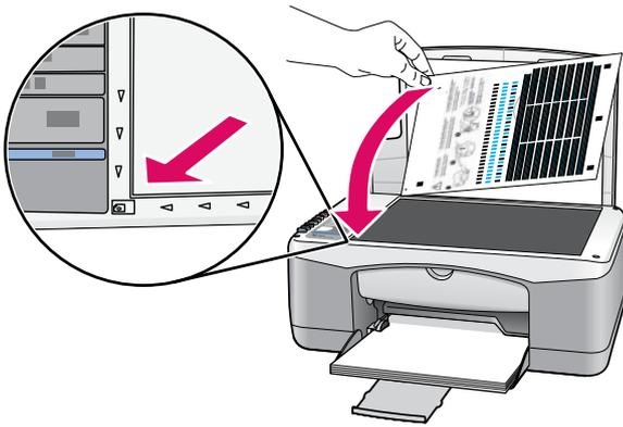
After the alignment page is printed, place it face down on the glass as shown in the picture. Close the lid.
