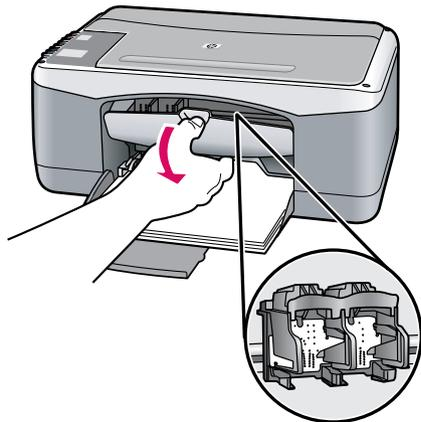
Open the print cartridge door. Wait until the print carriage moves to the center.
