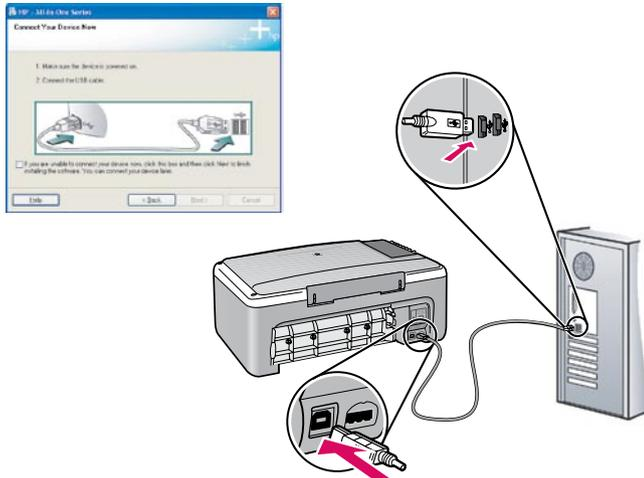
**Windows:** Once the USB prompt appears, connect the USB cable to the port on the back of the HP All-in-One, and then to any USB port on the computer.
