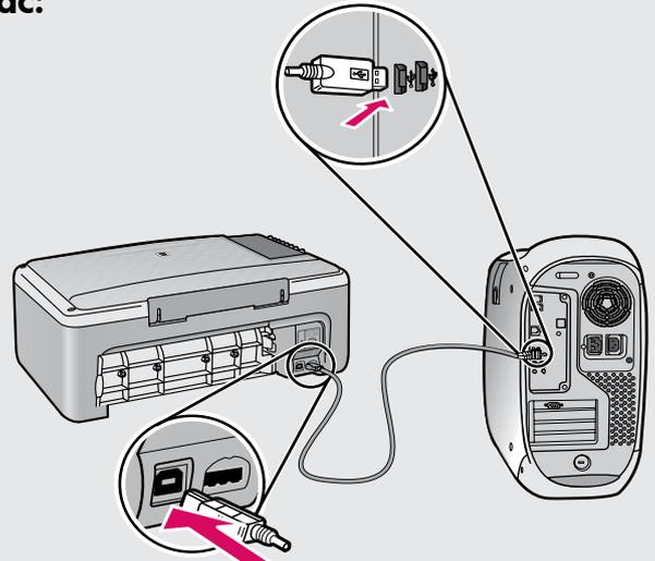
**Mac:** Connect the USB cable to the port on the back of the HP All-in-One, and then to any USB port on the computer.
