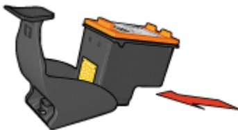
**To remove the print cartridge from the print cartridge protector**
