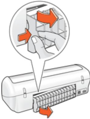
6. Remove the paper jam from the back of the printer, and then replace the rear access door securely.
