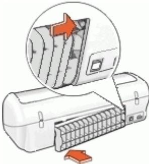
7. If the paper jam cannot be removed from the back of the printer, raise the printer cover, remove the paper jam from the front of the printer, and then lower the cover.
