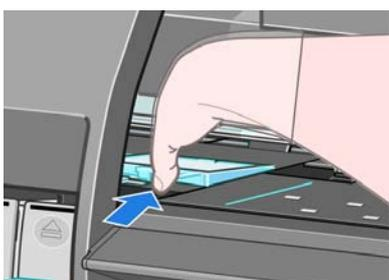
4. Push down on the tabbed edge until you hear the absorber click into place. Make sure that the top of the ink absorber is seated flatly and that none of the corners are higher than the plane of the platen.
