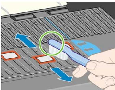
5. Use a clean, absorbent lint-free cloth that has been slightly dampened with isopropyl alcohol to wipe loosened ink deposits from the platen.
