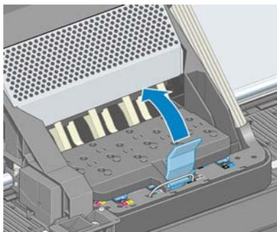
7. To remove a printhead, lift up the blue handle.
