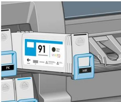
5. Lift the cartridge out of its drawer.
