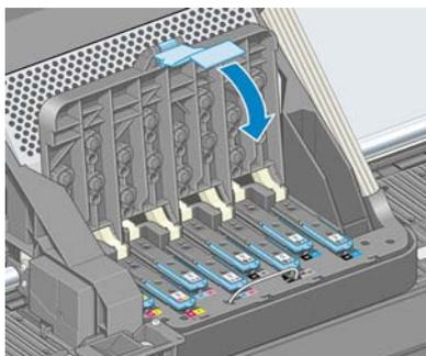
7. Make sure that the end of the blue handle catches the wire loop on the near side of the carriage.
