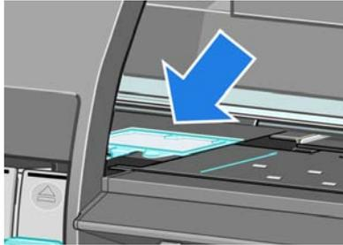
6. Lift the tab that extends from the front edge of the absorber.
