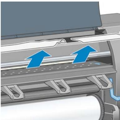
6. Carefully pull the remainder of the roll down and out of the printer.
