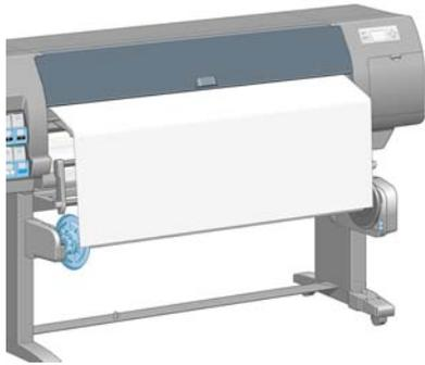
8. Pull the paper taut to the position shown in the following figure. Do *not* attempt to pull more paper out of the printer. Use tape to secure the paper to the spindle core. You might need to use more tape than is shown in the following image. The paper should be secure enough to support the weight of the loop-shaping core, which you insert in step 12.
