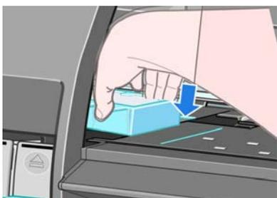
3. Use your thumb to slide the absorber to the back of the fitting in the spittoon.
