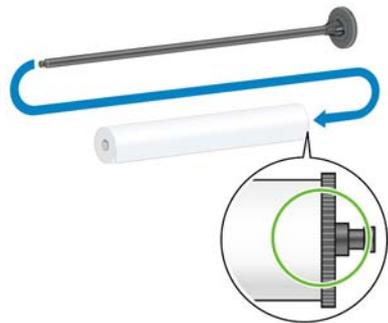
Make sure that the paper will wind off the roll in the correct direction. If it does not, remove the spindle from the roll, turn the roll 180° and rest it on the deflector. Then slide the spindle into the roll.
