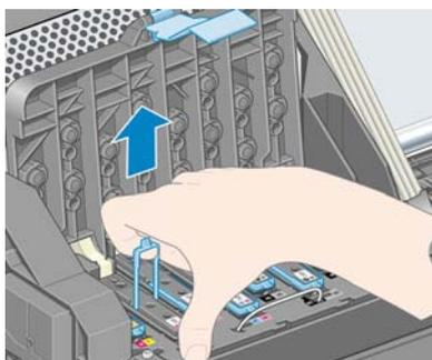
9. Gently pull the blue handle upward until the printhead is released from the carriage.
