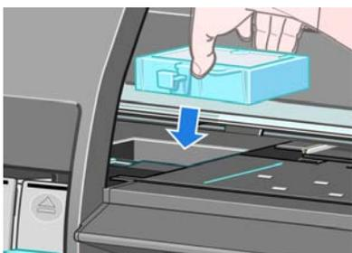
2. Insert the back edge of the absorber into the fitting in the spittoon.
