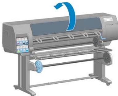
3. With a dry brush, remove ink deposits from the cutter groove.
