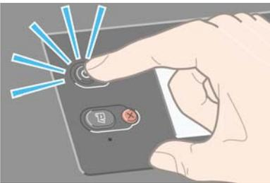
When you turn off the printer this way, the printheads are automatically stored with the maintenance cartridge, which prevents them from drying out.
