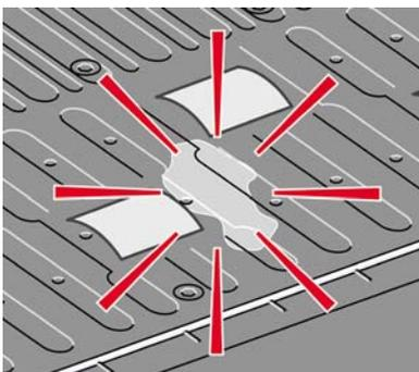
5. If oil spills onto the platen, wipe the platen clean by using the cloth that was supplied with the maintenance kit.
