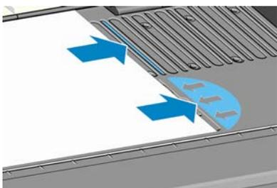
8. When the paper is correctly aligned with the blue line and half-circle, lower the paper-load lever.
