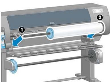
If you regularly use different paper types, you can change rolls more quickly if you pre-load rolls of different paper types on different spindles. Extra spindles are available for purchase.
