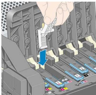
7. Rub the sponge against the contacts with a *light* force along the entire depth of the flex connector, inserting the wiper as far as allowed by the mechanical stop on the tool.
