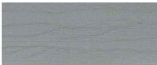
Aeroworms are wavy, horizontal bands produced by air-induced dot placement error (DPE). In extreme cases, aeroworms give the image a wood-grain appearance. The problem occurs most commonly on print jobs that are set for low-quality and high-speed. It does not occur when the custom print-quality setting is set to "best."
