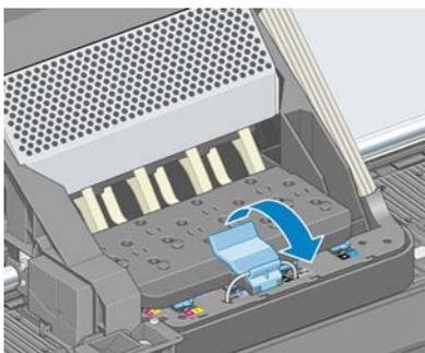
6. Lift up the cover. This provides access to the printheads.
