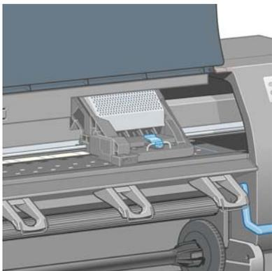
5. Pull up and release the latch on top of the carriage.
