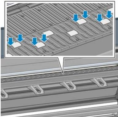
4. Put three drops of oil into each hole in the platen.
