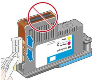
**CAUTION:** Do not touch the surface of the printhead that contains the nozzles, because the nozzles are easily damaged.
