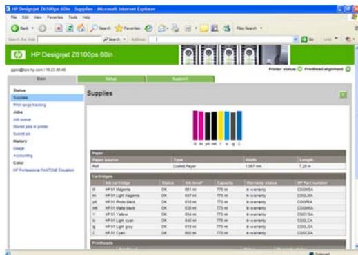
The Supplies page shows you the status of the ink cartridges (including the ink levels), the printheads, the maintenance cartridge, and the loaded paper.
