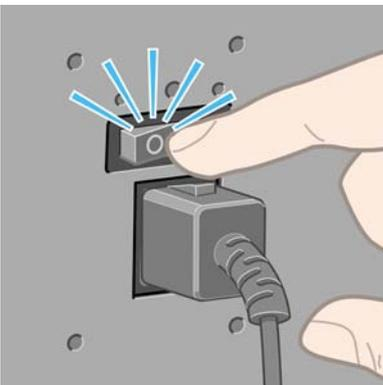
To turn it back on later, use the power switch at the rear, and then press the **Power** button.
