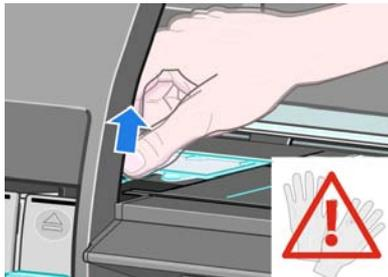
7. Lift the tab on the absorber until it is clear of the spittoon and you can easily grip the tab.
