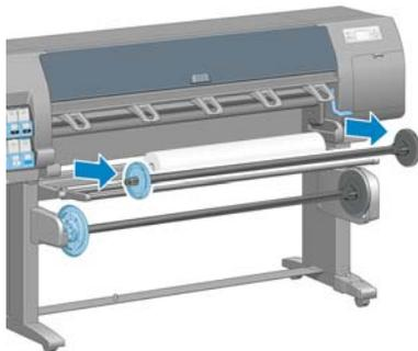
The spindle has a hub at each end to keep the roll in position. Remove the blue hub at the left end to mount a new roll. The hub slides along the spindle to hold rolls of different widths.
