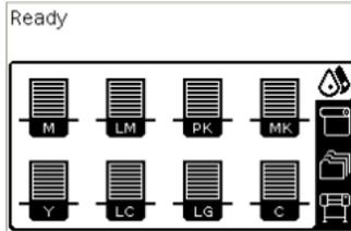
The front panel warns you when cartridge ink level is low. When a cartridge is empty, the printer stops printing and the front panel provides an explanation.
