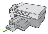
Securely snap the inkjet printable media onto the CD/DVD holder with the printable side up. The CD/DVD should be placed on the ring at the end of the holder with the arrows.
