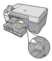
NOTE: The HP All-in-One pulls the CD/DVD holder while printing on the media. The CD/DVD holder might protrude about 7.5 cm (3 inches) at the back of the device. If the HP All-in-One is placed close to a wall, move it at least 3 inches away from the wall.
