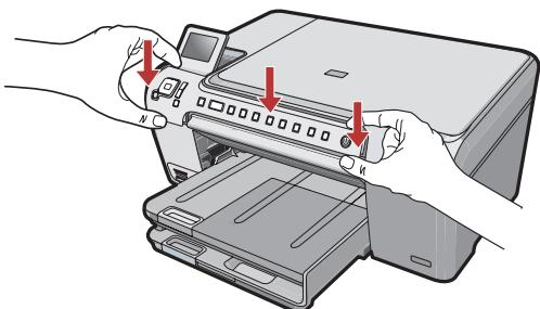
a. If the control panel faceplate is not already attached, position it over the buttons on the device.
