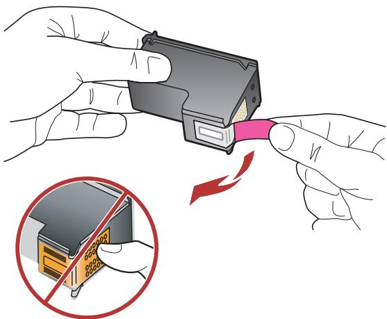
Remove the tape from both cartridges.
