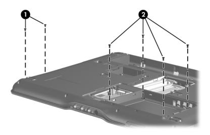
Removing the Top Cover Screws, Part 2
