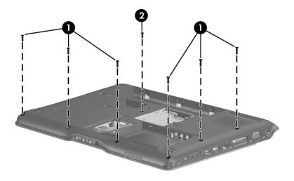
Removing the Top Cover Screws, Part 1
