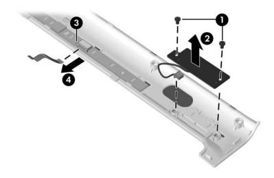
Removing the Power Button Board and LED Board Cable
