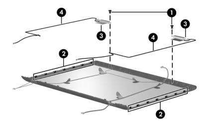
Removing the Wireless Antenna Transceivers and Cables
