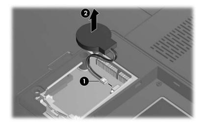
Replacing the RTC Battery
