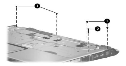
Removing the Top Cover Screws, Part 3
