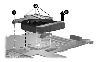
Removing Fan/Heat Sink Assembly
