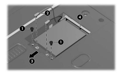
Removing a Mini Card Module
