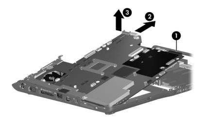
Removing the System Board
