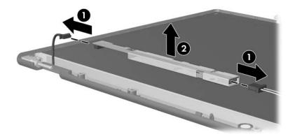
Removing the Display Inverter Board
