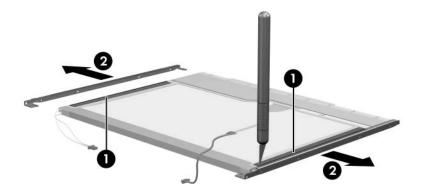
Removing the LCD Panel Frame
