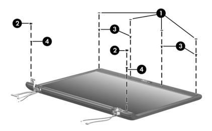
Removing the Display Bezel Screws
