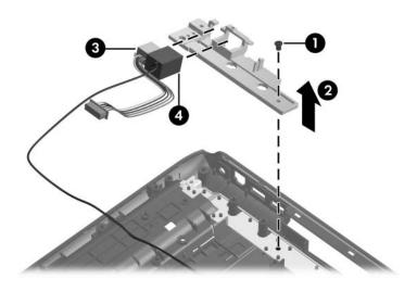
Removing the Power Connector Cable and Modem Cable
