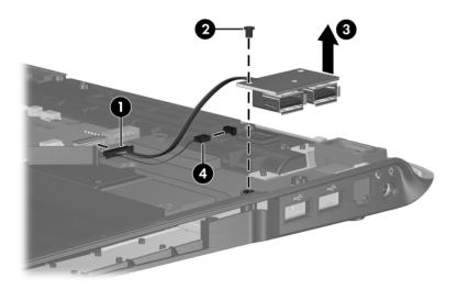
Removing the USB Board
