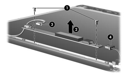
Removing the Display Inverter
