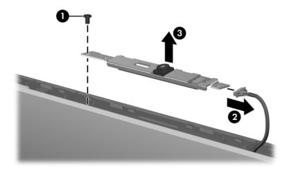
Removing the Display Web Camera
