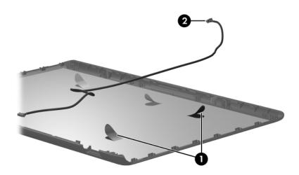
Removing the Web Camera Cable
