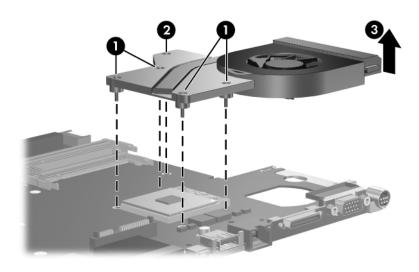
Removing Fan/Heat Sink Assembly
