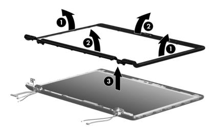
Removing the Display Bezel
