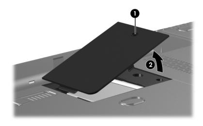
Removing the Mini Card Compartment Cover
