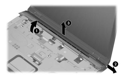
Removing the Switch Cover
