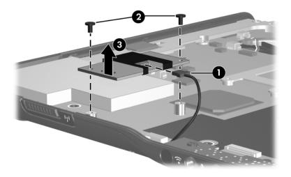
Removing the Modem Module
