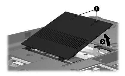
Removing the Memory Module Compartment Cover
