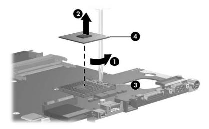
Removing the Processor
