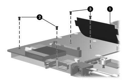
Removing the Fan/Heat Sink Assembly
