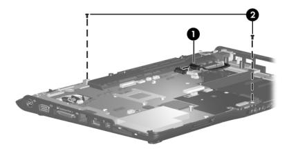
Removing the System Board Screws
