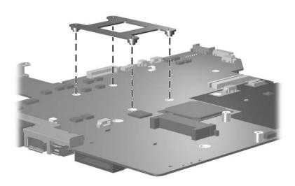
Removing the Fan/Heat Sink Assembly Mounting Bracket
