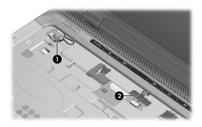
Disconnecting the Switch Cover Cables
