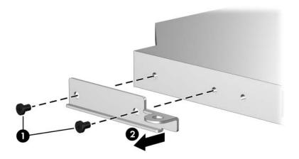
Removing the Optical Drive Bracket
