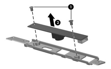
Removing the Display Web Camera Bracket
