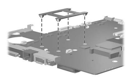
Removing the Fan/Heat Sink Assembly Mounting Bracket
