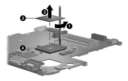
Removing the Processor
