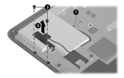
Removing the Wireless Switch Board
