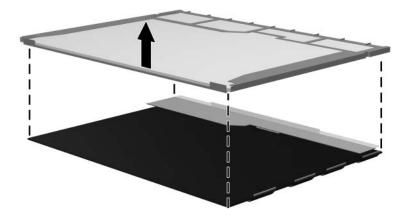
Removing the LCD Panel
