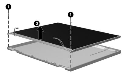
Removing the LCD Panel
