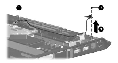
Removing the Display Lid Switch Module
