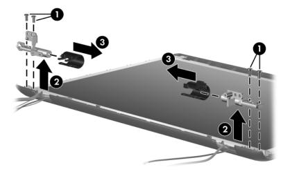
Removing the Display Hinges
