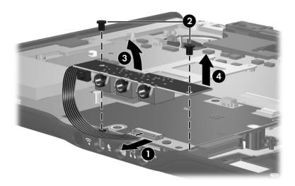
Removing the Audio/Infrared Board
