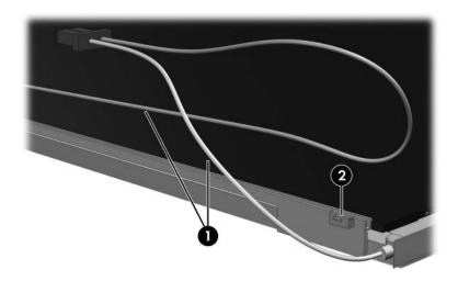
Releasing the Backlight Cables
