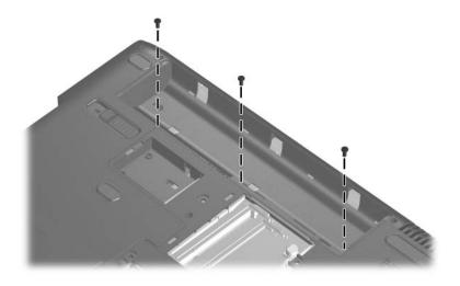
Removing the Keyboard Screws
