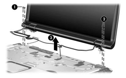
Removing the Display Assembly
