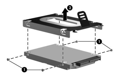
Removing the Hard Drive Frame and Connector
