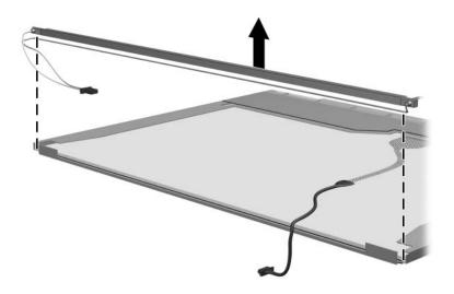
Removing the Backlight Frame
