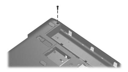
Removing the Display Screw
