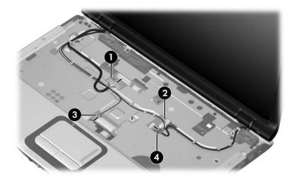
Disconnecting the Display, Web Camera, and Microphone Cables and Removing the Wireless Antenna Cables
