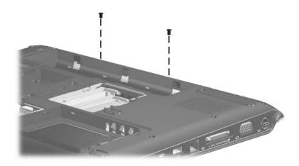
Removing the Base Enclosure Trim Screws
