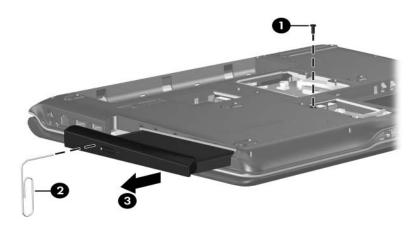
Removing the Optical Drive
