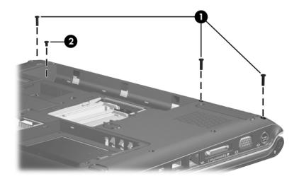
Removing the Switch Cover Screws
