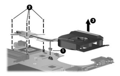
Removing the Fan/Heat Sink Assembly
