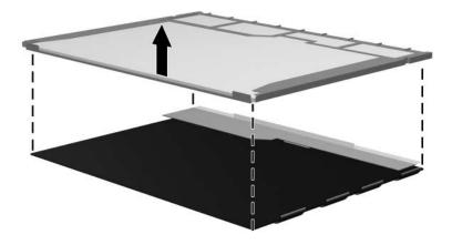
Removing the LCD Panel
