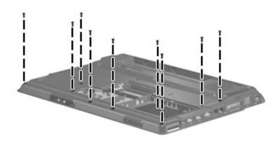
Removing the Top Cover Screws, Part 1
