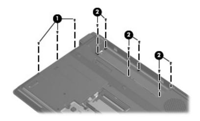
Removing the Top Cover Screws, Part 2
