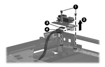
Removing the USB/Power Connector Board
