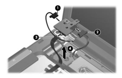
Removing the Power Button Board
