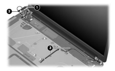
Disconnecting the Display Cables
