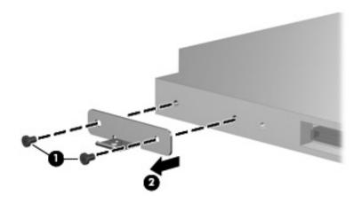
Removing the Optical Drive Bracket
