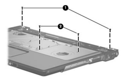
Removing the Top Cover Screws, Part 3
