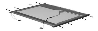
Removing the LCD Panel Frame Screws
