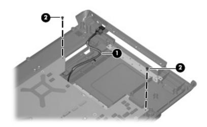
Removing the System Board Screws
