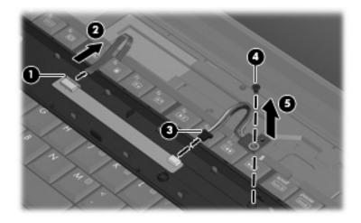
Removing the Num Lock Board
