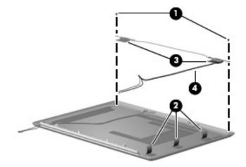
Removing the Wireless Antenna Transceivers and Cables
