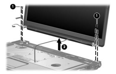
Removing the Display Assembly
