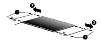
Removing the Display Hinges
