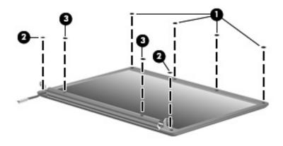
Removing the Display Bezel Screw Covers
