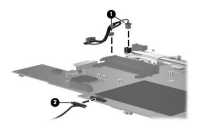
Removing the System Board Cables
