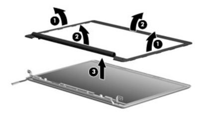
Removing the Display Bezel
