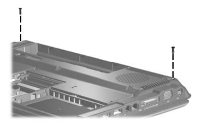
Removing the Switch Cover Screws
