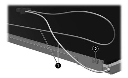
Releasing the Backlight Cables
