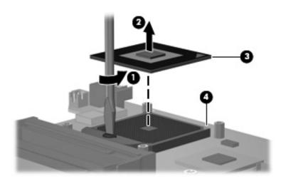
Removing the Processor
