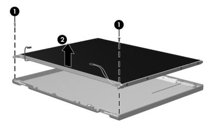
Removing the LCD Panel
