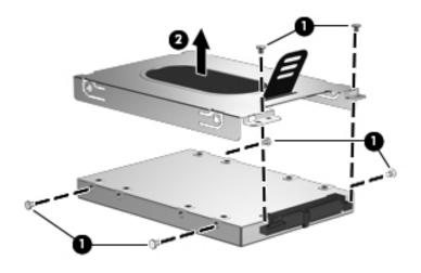
Removing the Hard Drive Bracket
