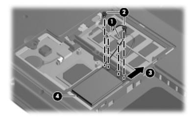
Removing a Mini Card Module
