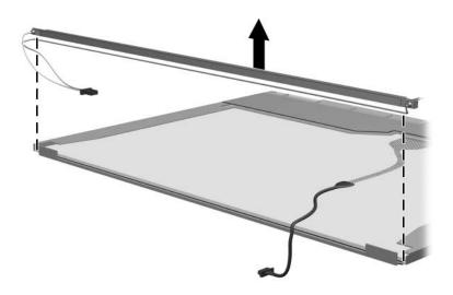
Removing the Backlight Frame
