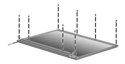
Removing the Display Bezel Screws
