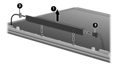
Removing the Display Inverter
