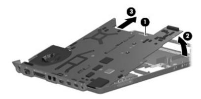
Removing the System Board
