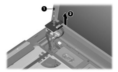
Releasing the Power Button Board
