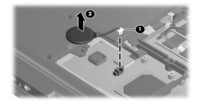
Removing the RTC Battery
