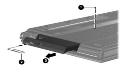
Removing the Optical Drive
