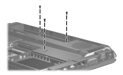
Removing the Keyboard Screws
