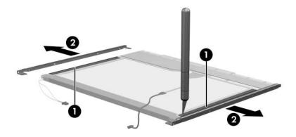
Removing the LCD Panel Frame
