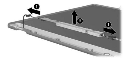
Removing the Display Inverter Board
