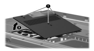
Removing the Memory Module Compartment Cover
