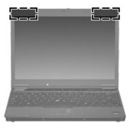
NOTE: For optimal transmission, keep the areas immediately around the antennae free from obstructions.
