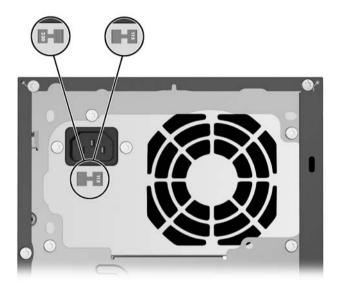
**CAUTION:** You should not need to change the voltage setting; however, you should verify that the voltage selection is compatible with your local power specifications. Failure to do so could result in damage to the computer.
