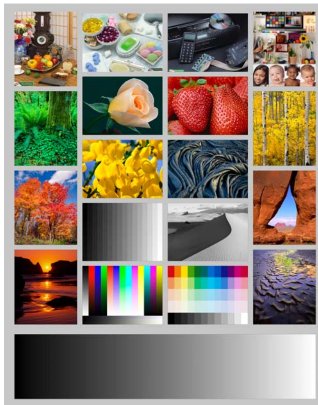
Figure: Bill Atkinson's test image used for a perceptual print quality test (this is a reduced size version, and converted from the original CIELAB color space to sRGB)
