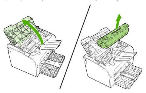
△ CAUTION: To prevent damage to the print cartridge, minimize its exposure to direct light.
