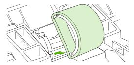
**6.** Rotate the top of the new pickup roller away from you until both sides snap into place.
