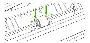
4. Gently pull the pickup roller up and out.
