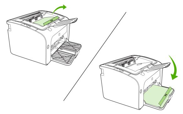
Click Continue to print side two. On the HP LaserJet P1505/P1505n, press Go on the device control panel after clicking Continue.
