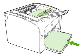
4. After side one has printed, without changing the orientation, remove the paper stack from the output bin. Do not discard blank sheets. Maintaining the same orientation, insert the paper stack into the priority feed tray or the main tray, printed side down.
