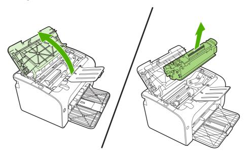
△ CAUTION: Do not touch the black-sponge transfer roller inside the device. Doing so can damage the device.
