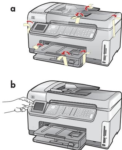
EN **a.** Remove all tape and protective film from the lid and from the front and back of the device.
