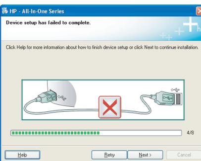
**EN** **Problem:** (Windows only) The **Device Setup Has Failed To Complete** screen appears.
