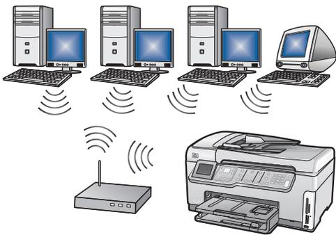
EN Use the instructions in **Section B** if you want a wireless (802.11b or 802.11g) connection between the HP All-in-One and your network. Equipment needed: wireless router.
