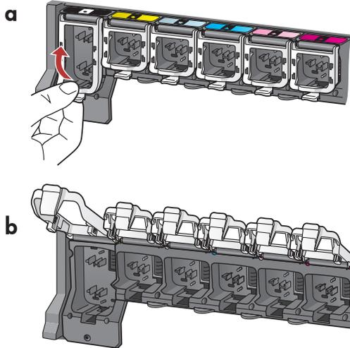
EN a. Squeeze the bottom of each latch to release it, and then lift the latch.
