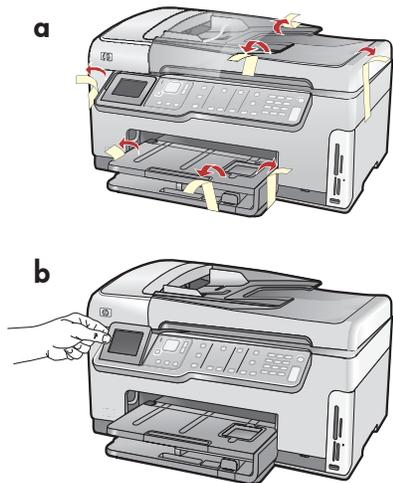
EN a. Remove all tape and protective film from the lid and from the front and back of the device. b. Lift the color graphics display and remove the protective film. You can adjust the angle of the display to a position suitable for viewing.
