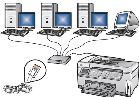
EN Use the instructions in **Section C** if you want an Ethernet cable connection between the HP All-in-One and your network. Equipment needed: router and Ethernet cable.
