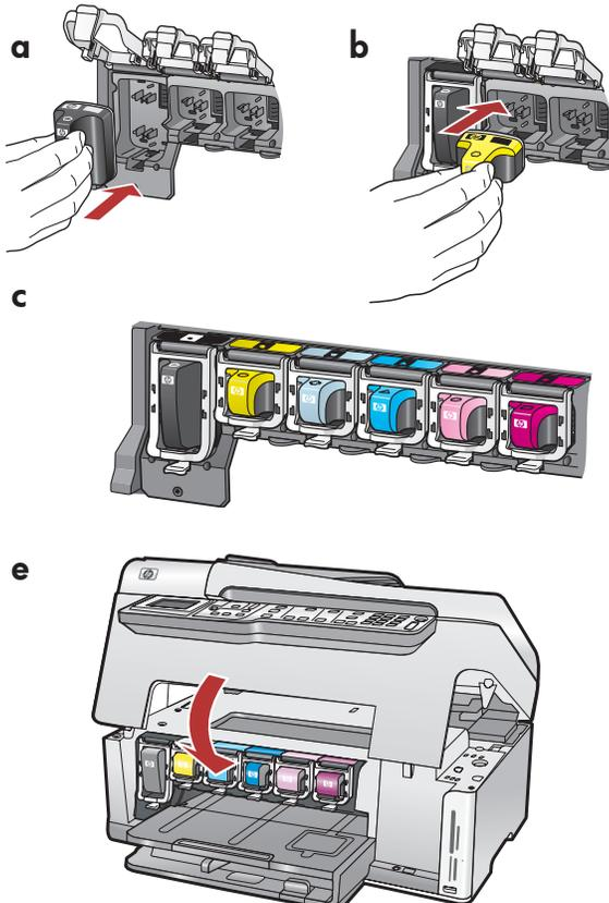
EN a. Match the color and pattern of the ink cartridge to the color and pattern above the latches.
