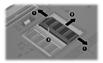
Reverse this procedure to install a memory module.
