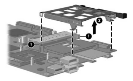
Reverse this procedure to install the PC Card assembly.
