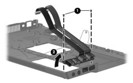
3. Remove the USB/audio board and cables from the base enclosure.
