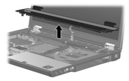
Reverse this procedure to install switch cover.
