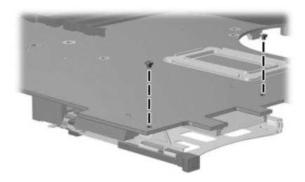
Where used: 2 screws that secure the PC Card assembly to the system board
