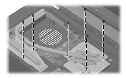
Where used: 6 screws that secure the heat sink to the system board
