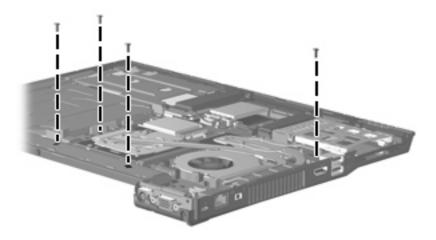
Where used: 4 screws that secure the system board frame to the base enclosure
