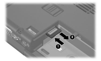
Reverse this procedure to install the SIM.
