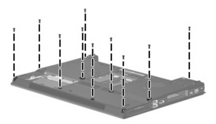
Where used: 10 screws that secure the top cover to the base enclosure
