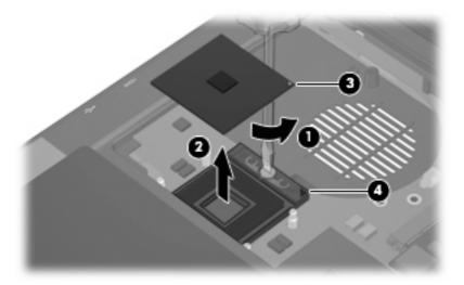
Reverse this procedure to install the processor.
