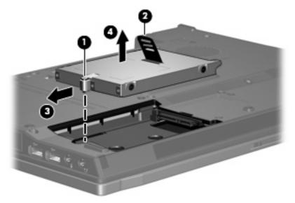
7. If it is necessary to replace the hard drive bracket, remove the two Phillips PM3.0×4.0 hard drive bracket screws (1) from each side of the hard drive.
