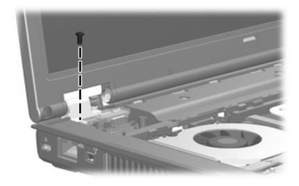
Where used: One screw that secures the display assembly to the computer
