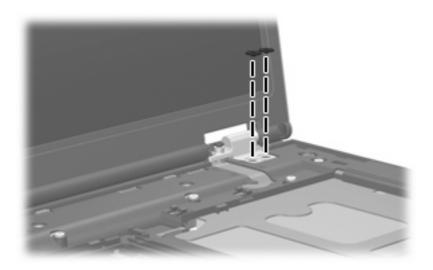
Where used: 2 screws that secure the display assembly to the computer
