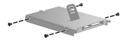
Where used: 4 screws that secure the hard drive bracket to the hard drive
