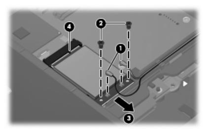
Reverse this procedure to install the WWAN module.
