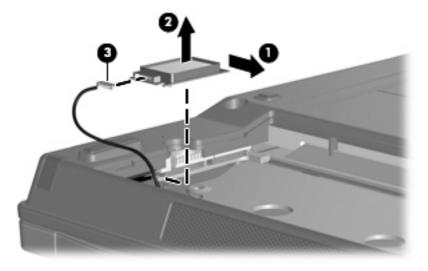
Reverse this procedure to reassemble and install the Bluetooth module.
