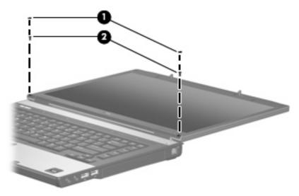
Flex the inside edges of the left and right sides (1) and the display bezel bottom edge (2) until the bezel disengages from the display assembly.
