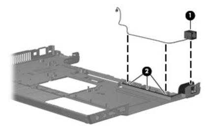
3. Remove the RJ-11 connector cable from the base enclosure.
