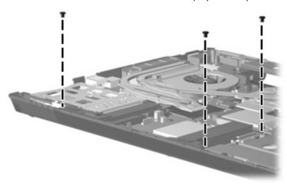
Where used: 3 screws that secure the speaker assembly to the base enclosure
