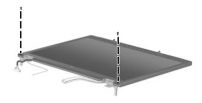
Where used: 2 screws that secure the display bezel bottom edge to the display enclosure
