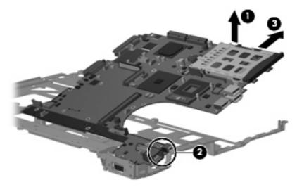
Reverse the preceding procedure to install the system board.
