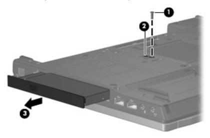
If it is necessary to replace the optical drive bracket, position the optical drive with the rear toward you.
