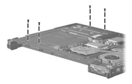
Where used: 4 screws that secure the system board frame to the base enclosure
