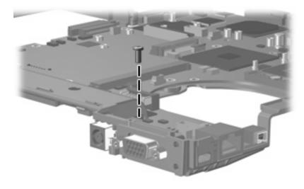
Where used: One screw that secures the system board to the system board frame
