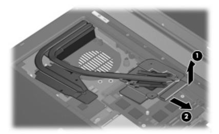
NOTE: The thermal material must be thoroughly cleaned from the surfaces of the heat sink (1) and (3), the processor (2), and graphics system component (4) each time the heat sink is removed. Thermal material is included with all heat sink and processor spare part kits.
