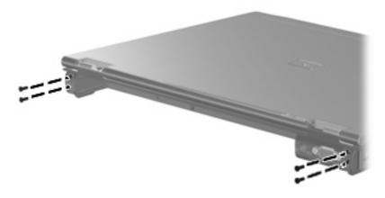
Where used: 4 screws that secure the display assembly to the computer
