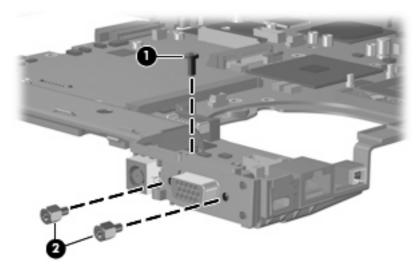
Lift the front edge of the system board (1) until the it clears the right side of the system board frame **(2)**.
