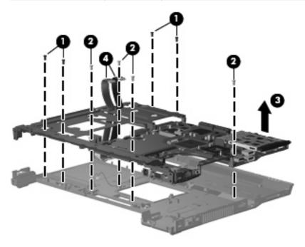
Remove the silver Phillips PM2.5 $\times$ 7.0 screw (1) and the two HM5.0 $\times$ 9.0 screw locks (2) that secure the system board to the system board frame.
