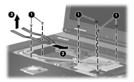
4. Lift the right side of the heat sink (1) to disengage it from the graphics card.
