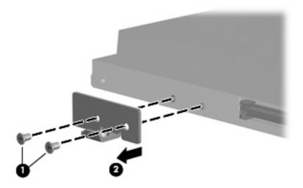
Reverse this procedure to install an optical drive.
