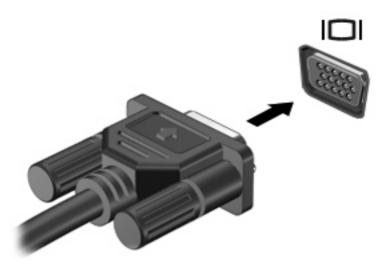
NOTE: If a properly connected external display device does not display an image, press fn+f4 to transfer the image to the device. Repeatedly pressing fn+f4 alternates the screen image between the computer display and the device.
