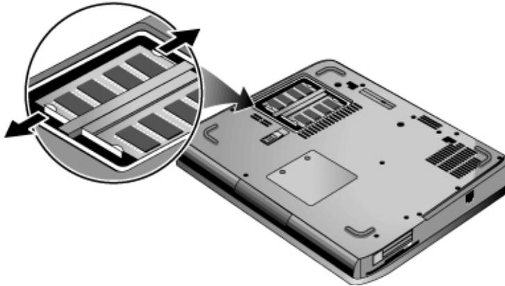
5. Pull the board out of the connector.
