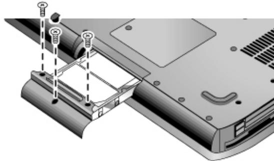
6. Gently slide the new drive into the hard drive compartment. Press firmly to make sure the connector seats properly.
