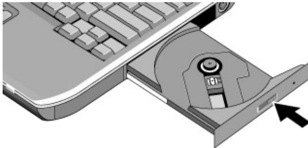
If your notebook loses power, you can manually open the drive to remove a CD. Insert a straightened paper clip into the recessed hole on the front of the drive to open it.
