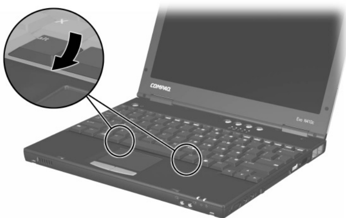
Figure 5-6. Releasing the Palm Rest
