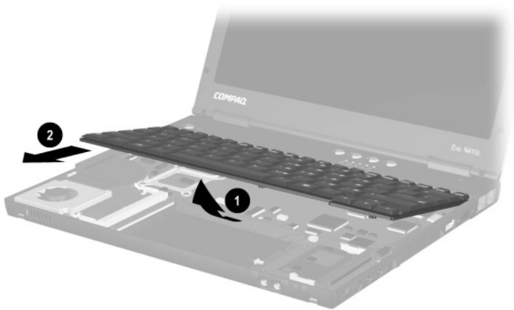
Figure 5-18. Releasing the Keyboard
