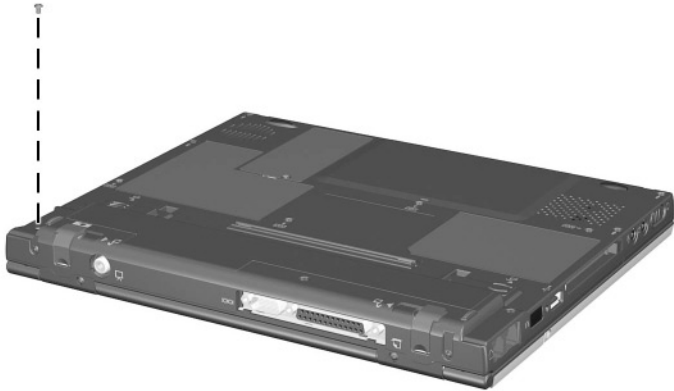
Figure C-7. TM2.0 x 4.0 Screw Location
