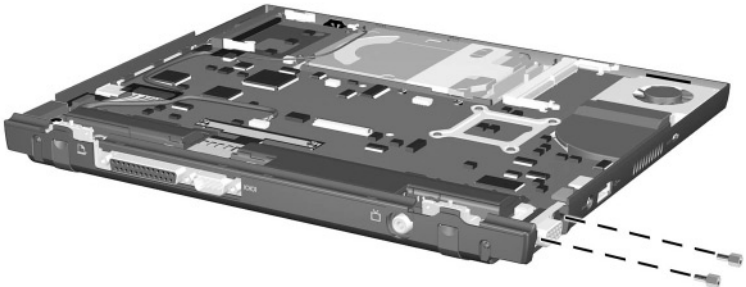
Figure C-10. HM5.0 × 9.5 Screwlock Locations
