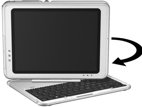
*Rotating the tablet PC toward the back of the keyboard*
