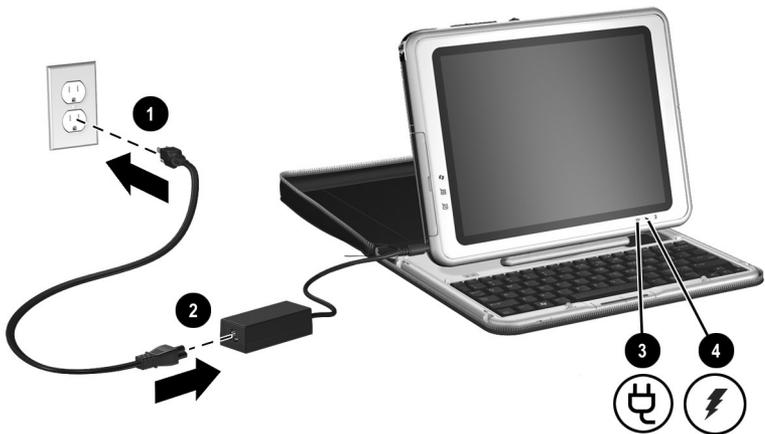
*Plugging the power cord into the AC adapter and an electrical outlet (AC adapters, power cords, and electrical outlets vary by region)*
