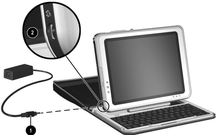
*Plugging the AC adapter cable into the AC power connector
