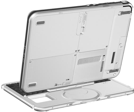
*Positioning the tablet PC and keyboard to detach the tablet PC*
