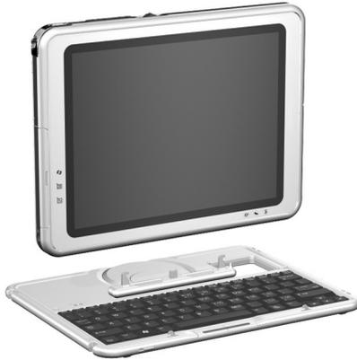
*Positioning the tablet PC above the keyboard*
