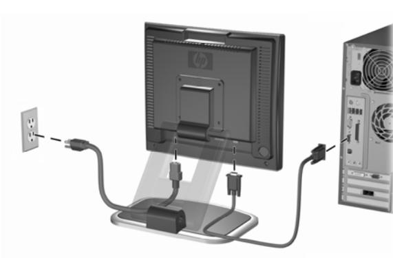
*Connecting the VGA Signal and Power Cable*
