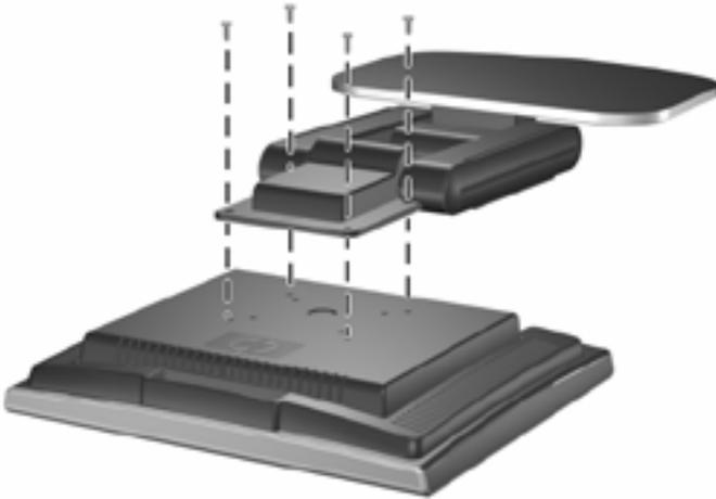
2. Mount the monitor to a swing arm or other mounting fixture by following the instructions included with the mounting fixture to be used.
