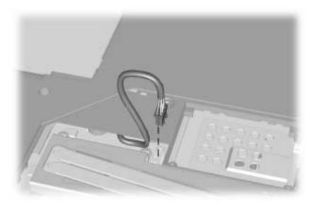
Figure 5-24. Disconnecting the Battery Terminal Cable
