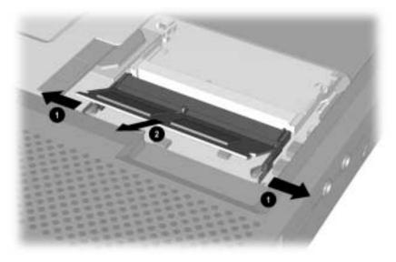
Figure 5-10. Removing a Memory Expansion Board
