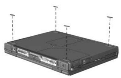
Figure 5-2. Installing the Computer Feet
