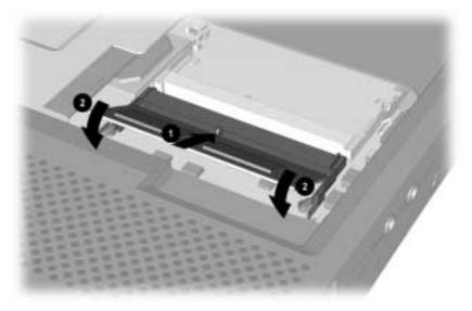
Figure 5-11. Installing a Memory Expansion Board
