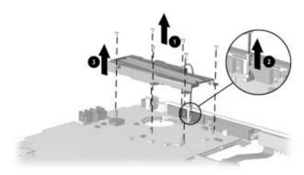
Figure 5-27. Removing the Fan and Heat Sink
