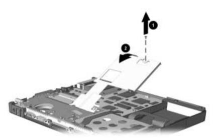
Figure 5-22. Removing the Front Shield
