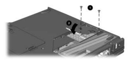
Figure 5-4. Installing a Modem or Modem/Network Interface Card
