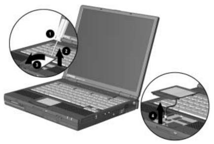
Figure 5-5. Removing the Touch Button
