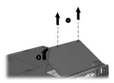
Figure 5-3. Removing the Mini PCI Slot Cover
