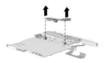
Figure 5-26. Removing the Voltage Converter Board
