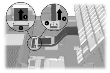
Figure 5-9. Releasing and Disconnecting the Keyboard Cables
