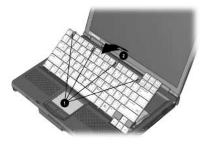
Figure 5-8. Releasing the Keyboard
