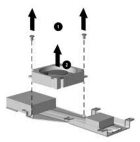
Figure 5-28. Removing the Fan
