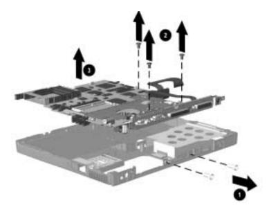
Figure 5-25. Removing the System Board
