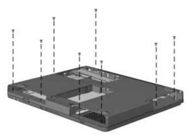
Figure 5-19. Removing the Top Cover Screws
