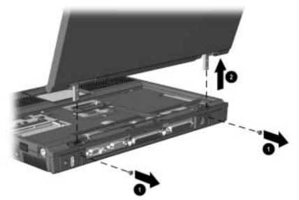
Figure 5-15. Removing the Display Assembly
