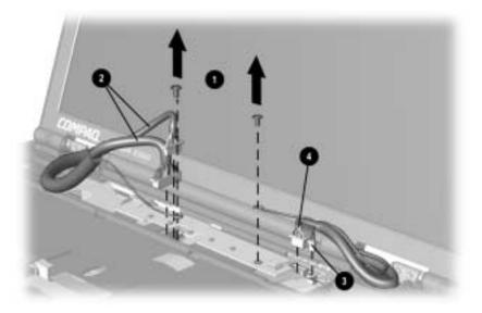
Figure 5-14. Disconnecting the Display Assembly Cables
