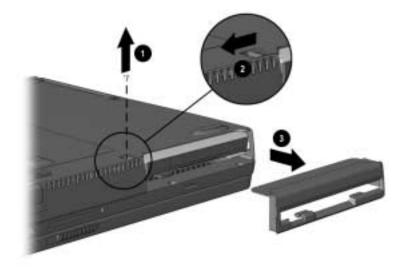
Figure 5-18. Removing the Diskette Drive Bezel
