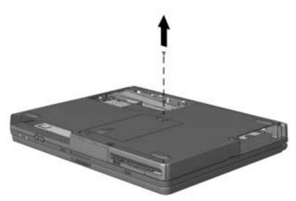
Figure 5-7. Removing the Keyboard Screw
