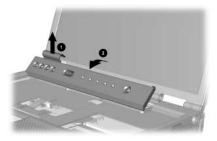
Figure 5-13. Removing the Switch Cover
