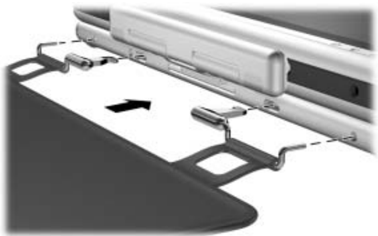
Attaching the screen protector to the keyboard
