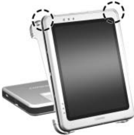
Snapping the tablet PC into place
