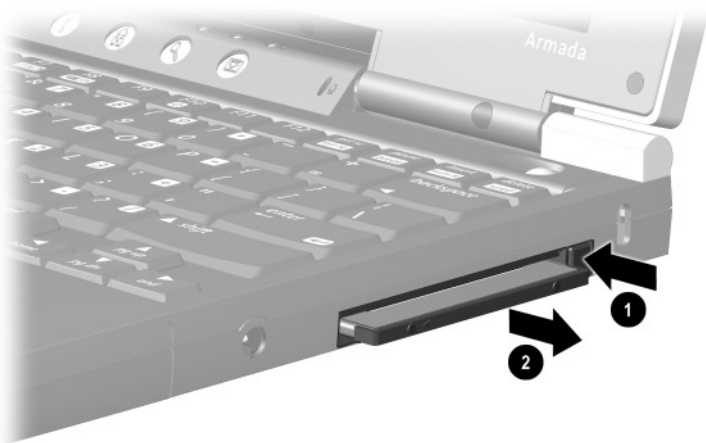
Removing a PC Card
