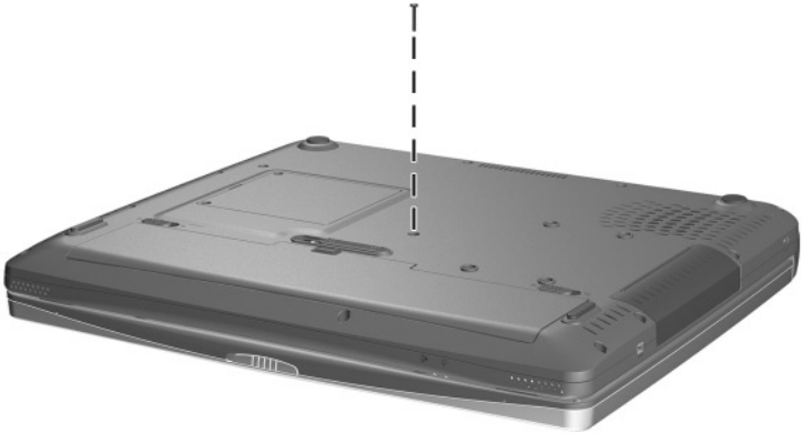
Figure C-8. Torx T8 M2.5 × 16.0 Screw Locations
