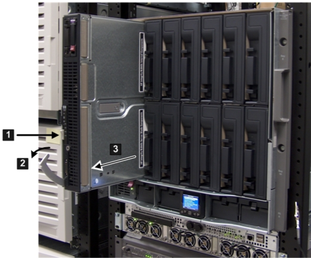
Figure 4-3 Removing the Server Blade from the Enclosure
