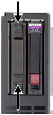
Figure 4-2 Removing a Disk Drive Blank
