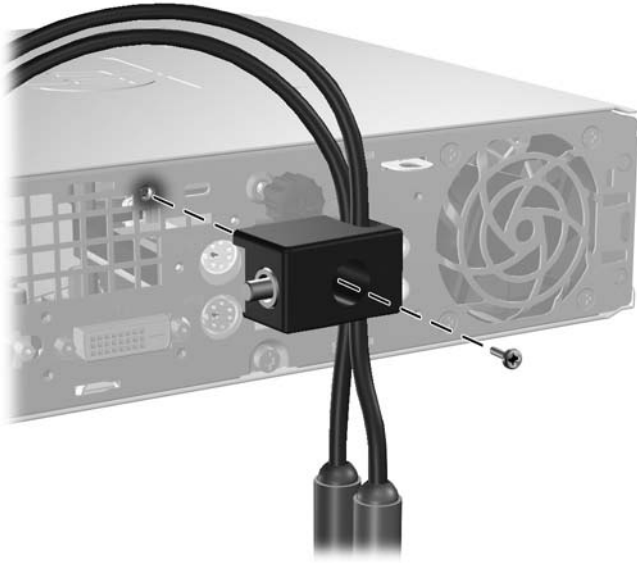
Figure C-6 Attaching the Lock to the Chassis
