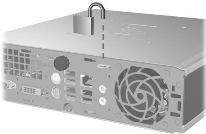
Figure C-3 Installing a Padlock
