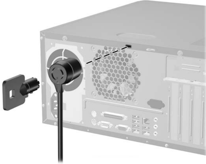
Figure 2-13 Installing a Security Lock
