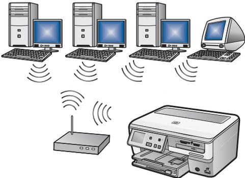
**EN** Use the instructions in **Section B** of this guide if you want a wireless (802.11b or 802.11g) connection between the HP All-in-One and your network. Equipment needed: wireless router.
