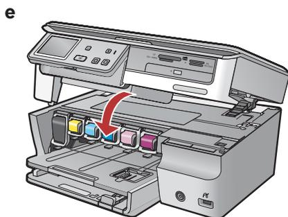
EN a. Match the color and pattern of the ink cartridge to the color and pattern above the latches.
