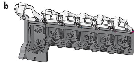
EN a. Squeeze the bottom of each latch to release it, and then lift the latch.
