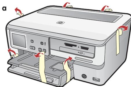
EN a. Remove all tape, and protective film from the lid and from the front and back of the device. b. Lift the color graphics display and remove the protective film. You can adjust the angle of the display to a position suitable for viewing.
