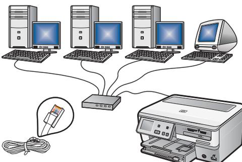
**EN** Use the instructions in **Section C** of this guide if you want an Ethernet cable connection between the HP All-in-One and your network. Equipment needed: router and Ethernet cable.
