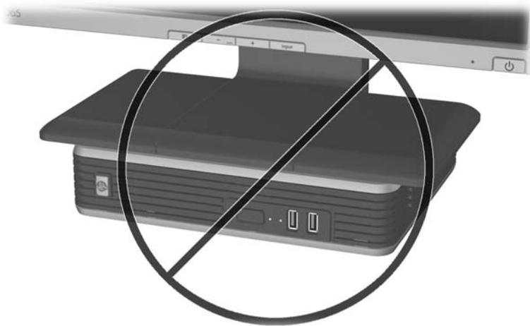
*Do not put a monitor on top of the thin client*
