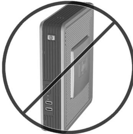
*Do not position the thin client vertically without using the stand*
