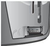
2. Remove the cap from the HP bt500 and insert it in the port.
