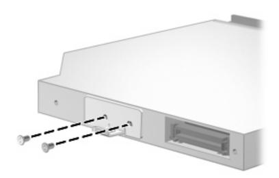
Where used: 2 screws that secure the optical drive bracket to the optical drive
