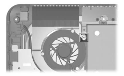
**Where used:** One captive screw (secured inside the video heat sink) that secures the system board and video board heat sink to the base enlcosure
