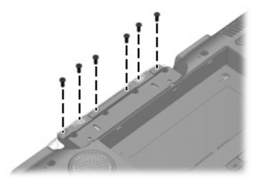
Where used: 6 screws that secure the display assembly to the computer
