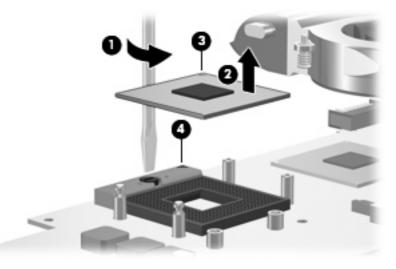
Reverse this procedure to install the processor.
