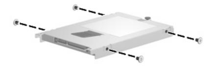
Where used: 8 screws that secure the hard drive brackets to the two hard drives
