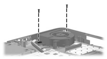
Where used: 2 screws that secure the processor fan to the base enclosure
