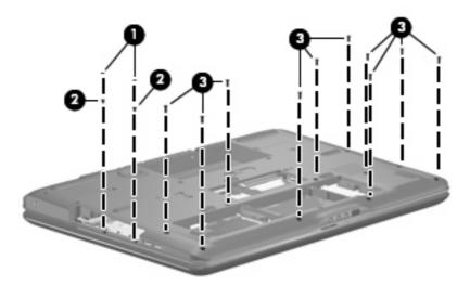
4. Remove the four Phillips PM2.5×5.0 screws (1) and the two Phillips PM2.5×11.0 screws (2) that secure the top cover to the computer.
