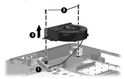
Reverse this procedure to install the processor fan.
