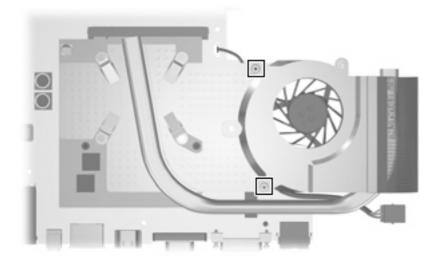
**Where used:** 2 captive screws (secured inside the video board heat sink) that secure the video board heat sink to the system board
