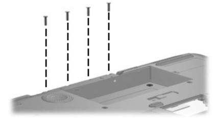
Where used: 4 screws that secure the rear cover to the computer
