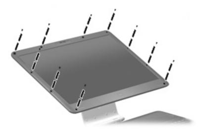
Where used: 10 screws that secure the display bezel to the display assembly
