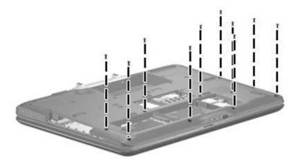
Where used: 10 screws that secure the top cover to the computer
