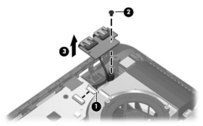
Reverse this procedure to install the rear USB board.
