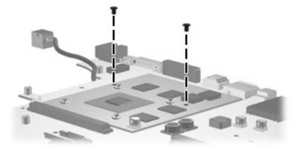
Where used: 2 screws that secure the video board to the system board
