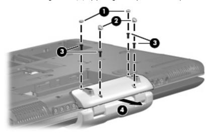
Reverse this procedure to install the hinge cover.
