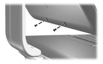
Where used: 2 screws that secure the display bezel to the display assembly
