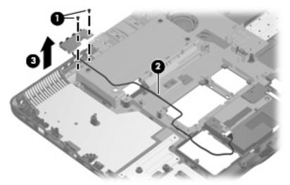
Reverse this procedure to install the audio connector board.
