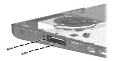
Where used: 2 screws that secure the system board to the base enclosure
