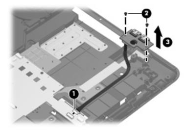
Reverse this procedure to install the front USB board.
