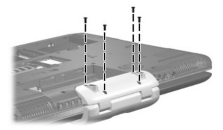
Where used: 4 screws that secure the hinge cover to the computer
