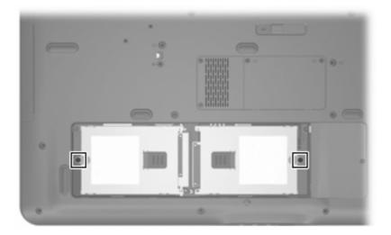
Where used: 2 captive screws (secured by C-clips) that secure the hard drives to the computer
