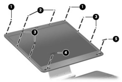
7. Remove the ten Phillips PM2.5×5.0 screws that secure the display bezel to the display assembly.
