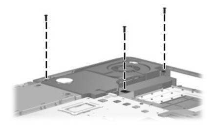
Where used: 3 screws that secure the subwoofer to the base enclosure
