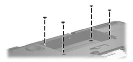
Where used: 4 screws that secure the rear cover to the computer
