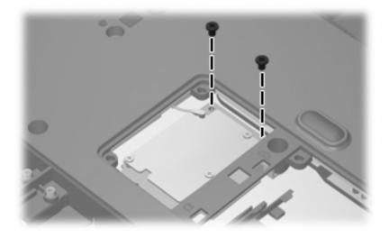
Where used: 2 screws that secure the TV tuner module to the system board
