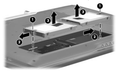
6. If it is necessary to replace the hard drive bracket, remove the four Phillips PM3.0×4.0 screws (1) that secure the hard drive bracket to the hard drive.
