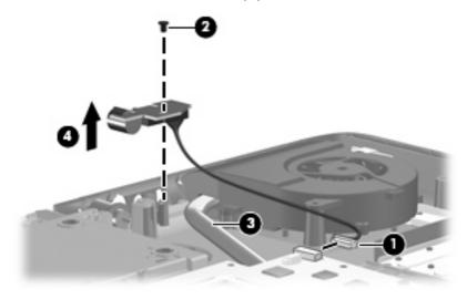
Reverse this procedure to install the video connector board.
