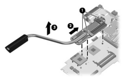
NOTE: The thermal material must be thoroughly cleaned from the surfaces of the processor heat sink (1) and the system board (2) each time the processor heat sink is removed. Thermal material must be installed on all surfaces before the processor heat sink is reinstalled. Replacement thermal material is included with all processor heat sink, system board, and processor spare part kits, and is also available using spare part number 413706-001.
