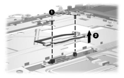
Reverse this procedure to install the TouchPad on/off board.
