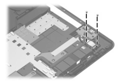
Where used: 2 screws that secure the Bluetooth module to the base enclosure
