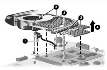
NOTE: The thermal material must be thoroughly cleaned from the surfaces of the video board components (1) and the video board heat sink (2) each time the video board heat sink is removed. Thermal material must be installed on all surfaces before the video board heat sink is reinstalled. Replacement thermal material is included with all video board heat sink and video board spare part kits, and is also available using spare part number 413706-001.
