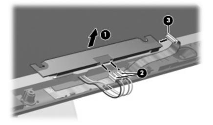
**16.** Remove the display inverter. The display inverter is available using spare part number 452308-001.
