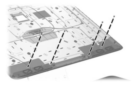
Where used: 4 screws that secure the speakers to the display enclosure
