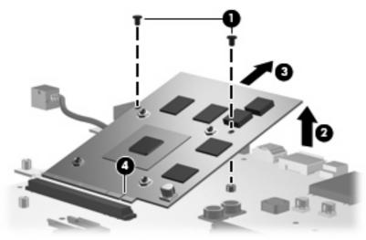
Reverse this procedure to install the video board.
