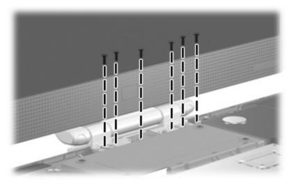
Where used: 6 screws that secure the display assembly to the computer
