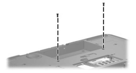
Where used: 2 screws that secure the top cover to the computer
