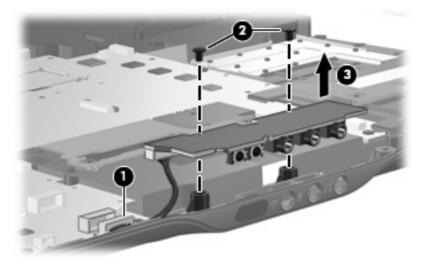
Reverse this procedure to install the audio/infrared board.
