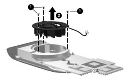
Reverse this procedure to install the video board fan.
