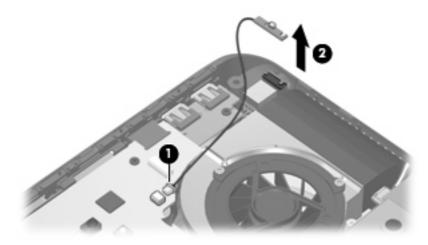
Reverse this procedure to install the power connector LED board.
