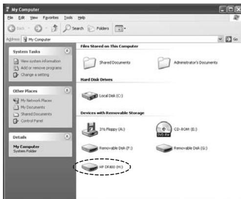
3 new drive letters will appear in Windows Explorer. These new drive letters represent the Digital Picture Frame's internal memory, Memory card slot 1 and Memory card slot 2. The digital picture frame will display the graphic below:
