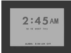
To change the clock time and alarm settings, press the
