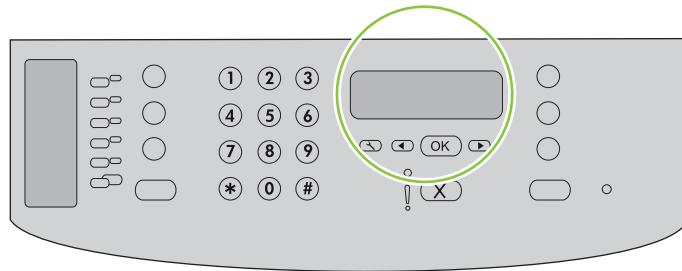
Use the alphanumeric buttons to enter the fax number and a company name or header. Press **OK**.
