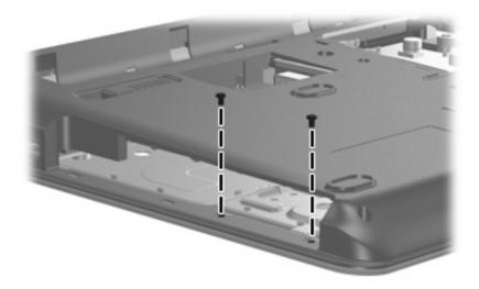
Where used: 2 screws that secure the top cover to the computer
