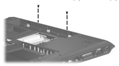
Where used: 2 screws that secure the top cover trim to the computer
