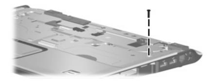
Where used: One screw that secures the top cover to the computer
