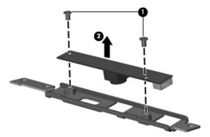
Reverse this procedure to install the camera module.
