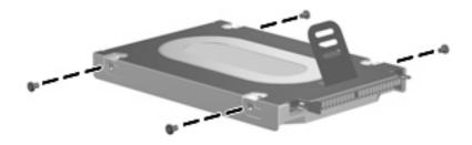
Where used: 4 screws that secure the hard drive bracket to the hard drive
