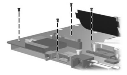
Where used: 4 screws that secure the ExpressCard assembly to the system board
