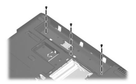
Where used: 3 screws that secure the keyboard to the computer
