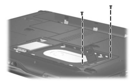
Where used: 2 screws that secure the hard drive to the computer
