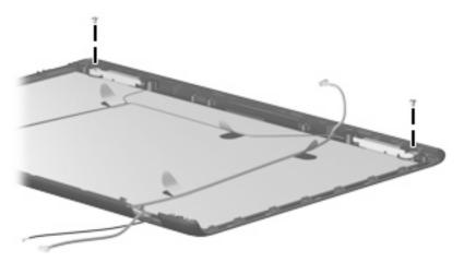
Where used: 2 screws that secure the wireless antenna transceivers to the display enclosure
