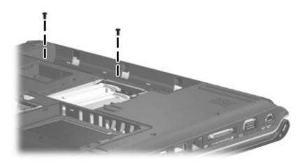
Where used: 2 screws that secure the switch cover to the computer
