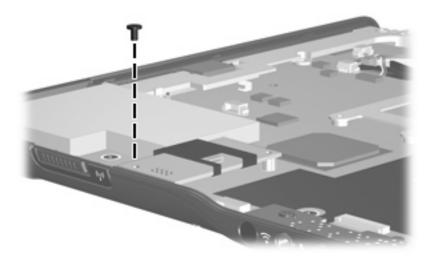
Where used: One screw that secures the modem module to the system board
