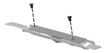
Where used: 2 screws that secure the camera module bracket to the camera module
