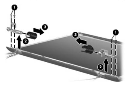
15. Remove the display panel from the display enclosure. The display panel is available using spare part number 448602-001 for computers with Intel processors, 448602-002 for computers with an Intel processor and a WWAN module, and 455810-001 for computers with AMD processors.
