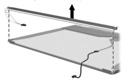
**WARNING!** The backlight contains mercury. Exercise caution when removing and handling the backlight to avoid damaging this component and causing exposure to the mercury.
