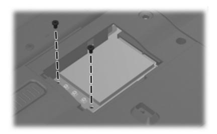
Where used: Two screws that secure the WLAN module to the computer
