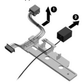
Reverse this procedure to install the power connector cable and modem cable.
