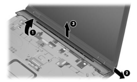
Reverse this procedure to install the switch cover.
