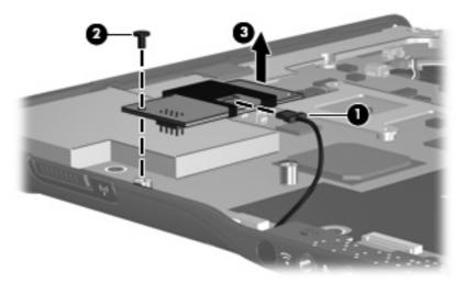
4. Remove the modem module.
