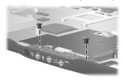
Where used: 2 screws that secure the audio board to the computer
