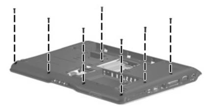
Remove the two Phillips  $PM2.0\times3.0$  screws (1) and the three Phillips  $PM2.0\times4.0$  screws (2) that secure the top cover to the computer.
