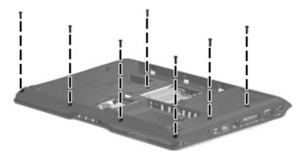
Where used: 7 screws that secure the top cover to the computer
