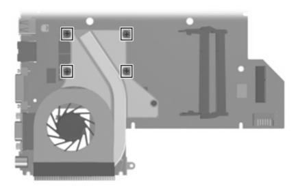
**Where used:** 4 captive screws (secured by C-clips) that secure the fan/heat sink assembly to the system board
