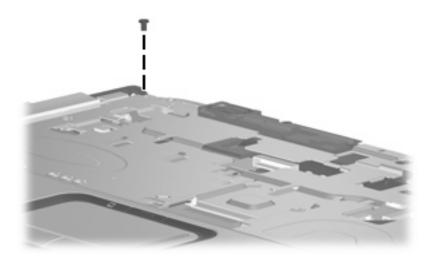
Where used: One screw that secures the top cover to the computer
