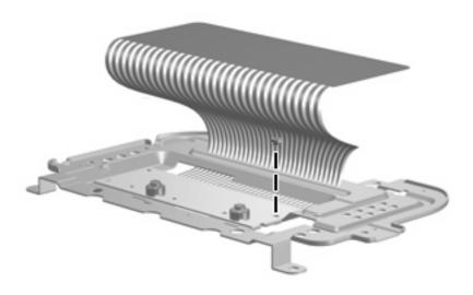
Where used: One screw that secures the TouchPad bracket to the TouchPad board
