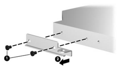
Reverse the above procedure to reassemble and install the optical drive.
