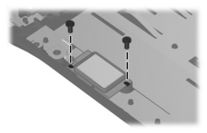
Where used: 2 screws that secure the Bluetooth module to the computer
