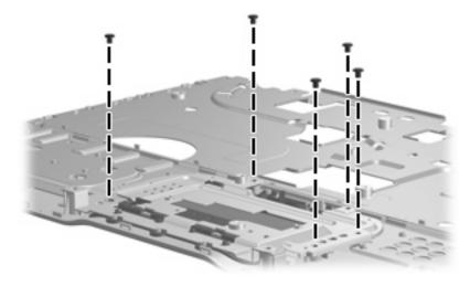
Where used: 5 screws that secure the TouchPad to the top cover
