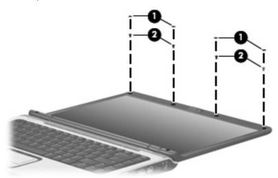
Flex the inside edges of the left and right sides (1) and the top edge (2) of the display bezel until the bezel disengages from the display enclosure.
