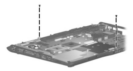
Where used: 2 screws that secure the system board to the computer
