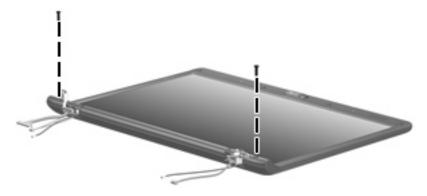
Where used: 2 screws that secure the display bezel bottom edge to the display assembly
