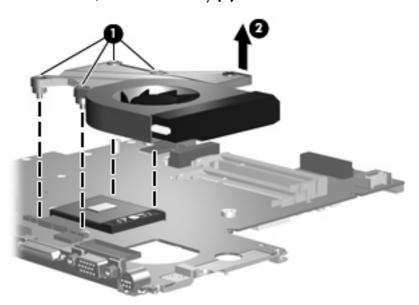
NOTE: The thermal material must be thoroughly cleaned from the surfaces of the fan/heat sink assembly (1) and (2), and (3), the system board components (4) and (6), and the processor (5) each time the fan/heat sink assembly is removed. Thermal pads and thermal paste must be installed on all surfaces before the fan/heat sink assembly is reinstalled. Thermal pads and thermal paste are included with all fan/heat sink assembly, system board, and processor spare part kits.
