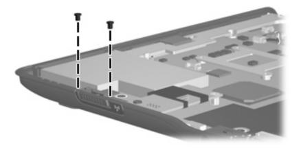
Where used: 2 screws that secure the wireless switch board to the computer
