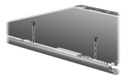
Where used: 2 screws that secure the display inverter to the display enclosure
