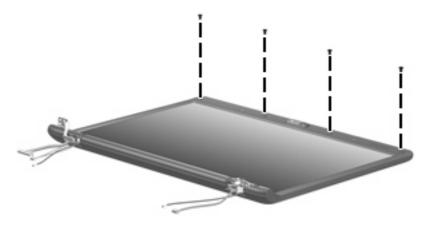
Where used: 4 screws that secure the display bezel top edge to the display assembly
