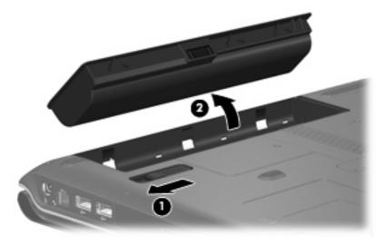
To insert the battery, insert the rear edge of the battery into the battery bay and pivot the front edge downward until the battery is seated. The battery release latch automatically locks the battery into place.
