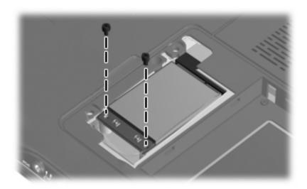
Where used: Two screws that secure the WWAN module to the computer
