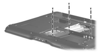
Where used: 3 screws that secure the top cover to the computer
