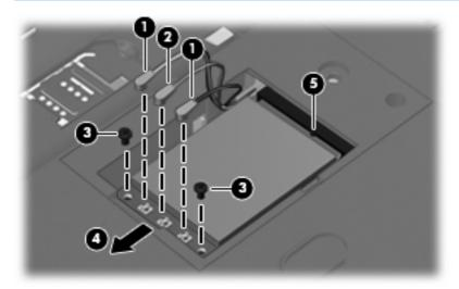
Reverse this procedure to install a WLAN module.
