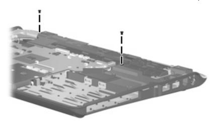
Where used: 2 screw that secures the speaker assembly to the computer
