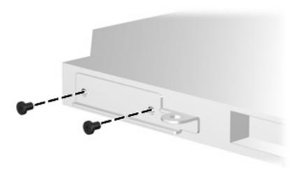
Where used: 2 screws that secure the optical drive bracket to the optical drive
