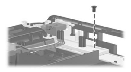
Where used: One screw that secures the connector bracket to the computer
