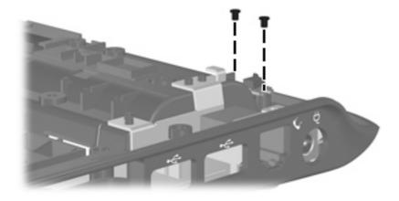
Where used: 2 screws that secure the display switch module to the computer
