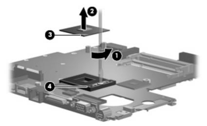
Reverse this procedure to install the processor.
