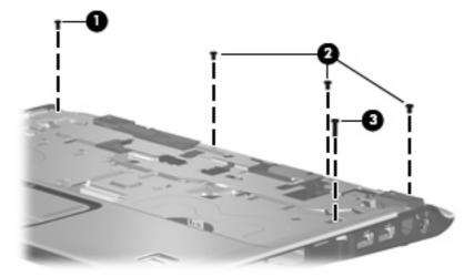
Lift the front edge of the top cover and remove it.
