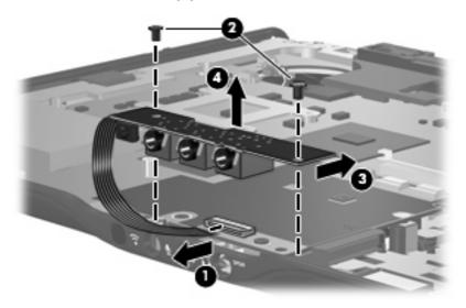
Reverse the above procedure to install the audio board.
