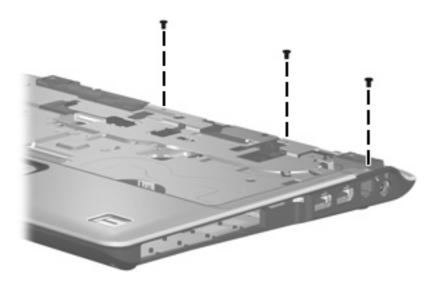
Where used: 3 screws that secure the top cover to the computer
