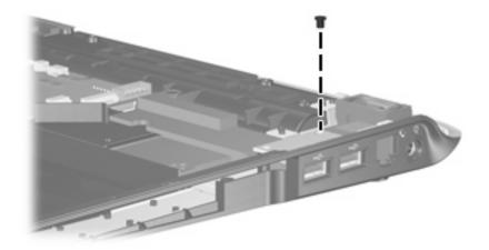
Where used: One screw that secures the USB board to the computer
