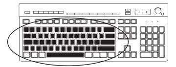
The alphanumeric keys are the main keys found on a standard typewriter.
