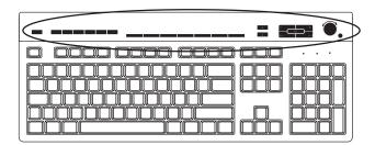
There are special buttons (select models only) at the top of the keyboard. These buttons operate a CD or DVD player, control speaker volume, connect you to the Internet, or provide quick access to specific functions. (Some keyboard models have some of these special buttons to the left side of the main keys, some do not have the Internet buttons, and some use a different layout on the top right.)
