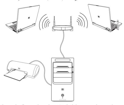
The preceding illustration shows a home LAN. The desktop computer has a wired connection to a wireless router. The desktop computer also has a printer that it shares with the other computers on the network. Each notebook computer has a wireless connection to the network router.
