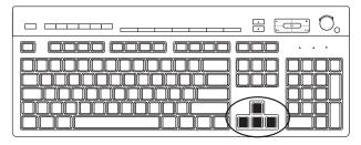
The arrow keys are controls for moving up, down, right, and left. You can use these keys instead of the mouse to move the cursor for navigation on a Web page, in a document, or in a game.
