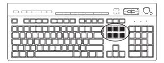
The edit keys are Insert, Home, Page Up, Delete, End, and Page Down. Use these keys to insert and delete text, and to quickly move the cursor on the screen. The edit keys function differently with some software programs.
