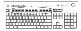
The function keys, located above the main keys, are labeled F1 through F12. Most function key operations vary by software program. F1 and F3 are available at all times:
