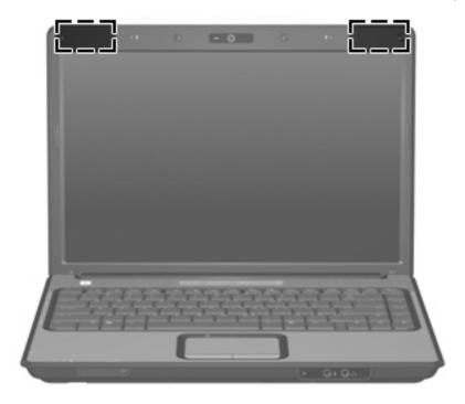
NOTE: For optimal transmission, keep the areas immediately around the antennae free from obstructions.
