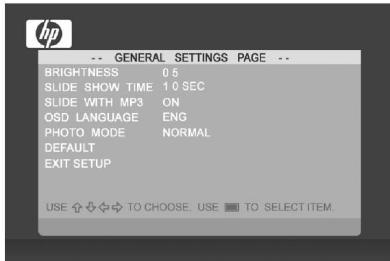
**BRIGHTNESS:** Adjust brightness from -10 to +10
