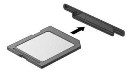
When you insert a digital card, you will hear a sound when the device has been detected, and a menu of available options may be displayed.
