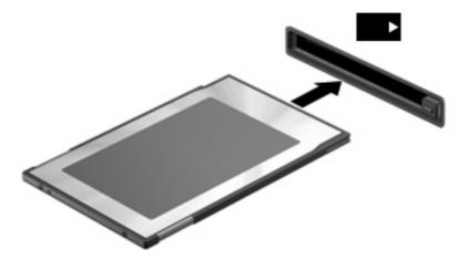
When you insert a PC Card, you will hear a sound when the device has been detected, and a menu of available options may be displayed.
