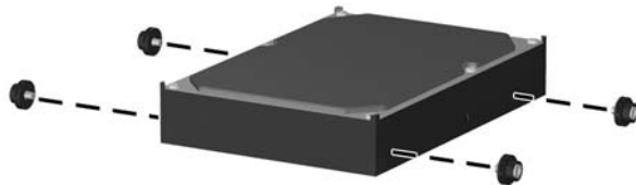
Figure 2-28 Installing Hard Drive Guide Screws
