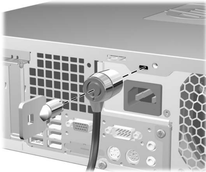
Figure C-1 Installing a Cable Lock
