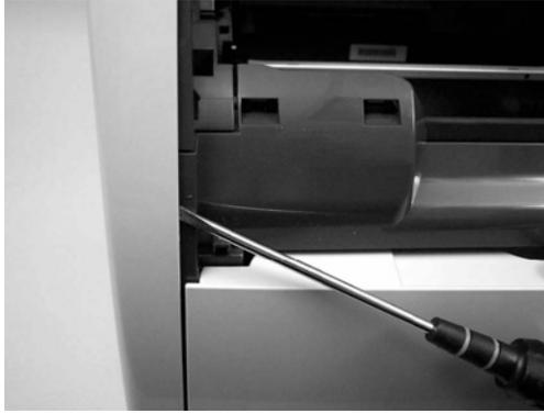
**Disengage latch at front of printer**
