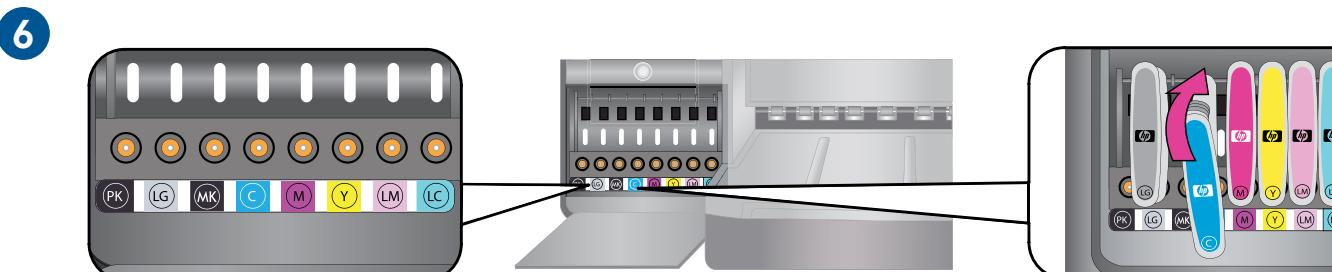
Insert all eight ink cartridges into their color-coded stalls. Press firmly on each cartridge until it snaps into place.
