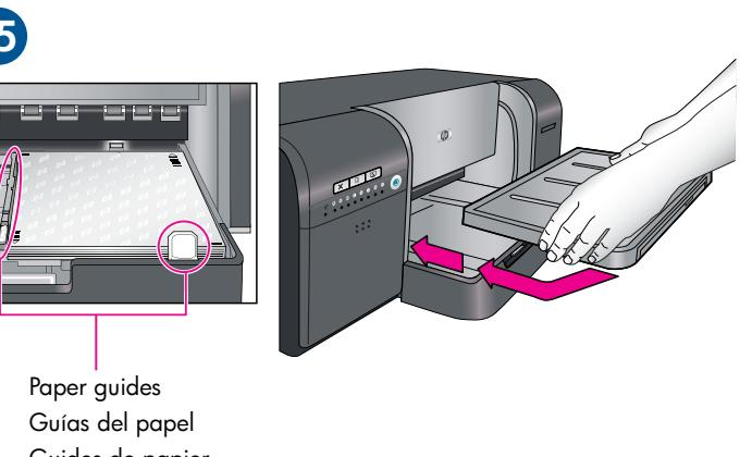
Adjust the paper guides. Check that the paper is lying flat. Slide the output tray back into place.
