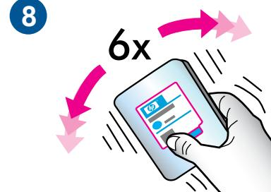
Shake each printhead well (six times) before unwrapping it.
