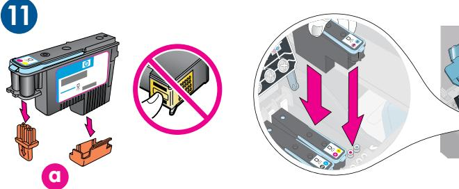
Open each printhead package, and remove and discard the orange caps (a). Do not touch the gold-colored contacts. Insert each printhead into its color-coded stall, pressing firmly until the printhead snaps into place (b).
