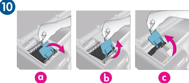
Pull the blue handle forward (a), then lift it up (b) and move it back (c).
