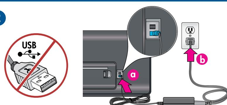
**Windows users: Do not connect the USB cable until prompted by the software install program (step 17).** Connect the power cord to the printer (a), and then to a power outlet (b). The printer turns on automatically.
