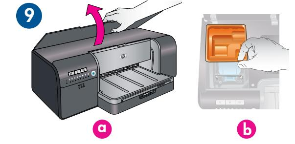
Open the top door (a). Remove orange plastic restraint (b). **Save the restraint for transporting the printer.**
