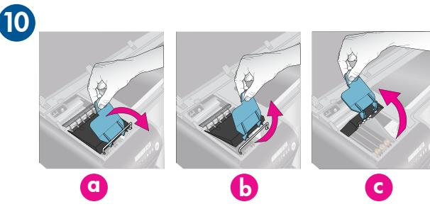
Pull the blue handle forward (a), then lift it up (b) and move it back (c).
