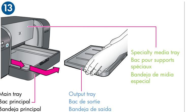
Remove the **output tray** straight out, by pulling it firmly. The output tray is the removable 'lid' on top of the main tray.
