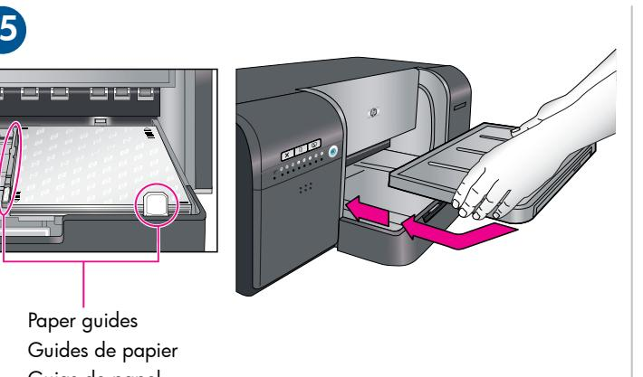
Adjust the paper guides. Check that the paper is lying flat. Slide the output tray back into place.
