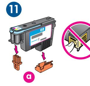
Open each printhead package, and remove and discard the orange caps (a). Do not touch the gold-colored contacts. Insert each printhead into its color-coded stall, pressing firmly until the printhead snaps into place (b).
