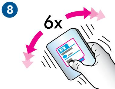
Shake each printhead well (six times) before unwrapping it.
