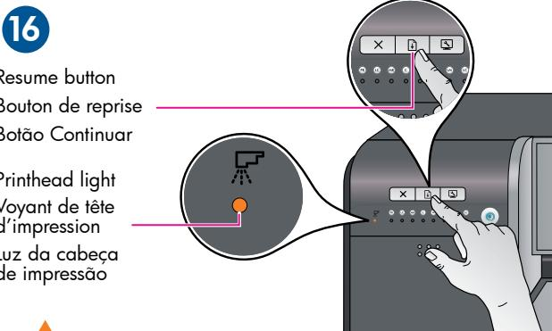
**IMPORTANT** Press the **Resume button** [ ] to start printer calibration. Calibration takes 30–40 minutes. Use this time to install the software (step 17). When the **Printhead light** [ ] goes off, calibration is complete.
