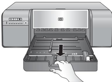
**💡 TIP:** You can remove the tray from the printer, if necessary, by grasping the sides of the tray with both hands and pulling it towards you.
