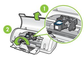
Insert print cartridges. Push cartridges forward until they 'click' into place.
