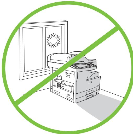
To position the device, select a sturdy, well-ventilated, dust-free area that is out of direct sunlight.
