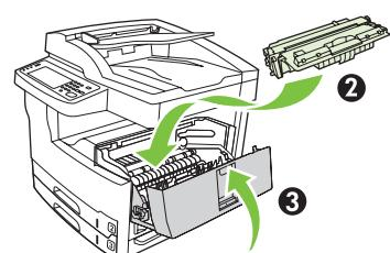
**5) Open the upper-right door and remove the orange print-cartridge locks.**
