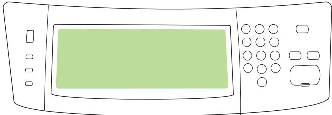
**18) Configure the IP address (if necessary).** On the control panel, scroll to and touch **Administration**. Scroll to and touch **Initial Setup**, and then **Networking and I/O**. Touch **Embedded Jetdirect**, **TCP/IP**, and **IPV4 Settings**. Touch **Manual Settings**, and then enter the **IP Address**, **Subnet Mask**, and **Default Gateway**.
